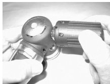
Fig. 132 -INSTALLING A TRT ON A REGULATOR
