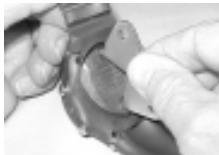
Fig. 113A - BATTERY HATCH REMOVAL (Tool)
