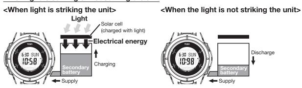
The TUSA IQ 1203 CE, when charged, will always display the clock feature, even if no light is present. On land, the computer is making calculations every 20 sec. In Dive Mode (submersed), the computer is making calculations every second.
