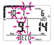
The DECO information and the DECO icon will blink continuously. The warning will operate twice for three seconds.
