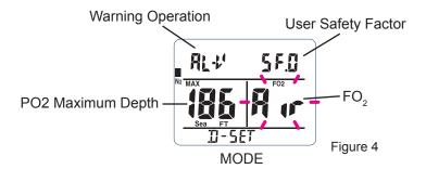
Use the dive set mode to set the oxygen concentration (FO<sub>2</sub>), user safety function (SF), warning alarm sound or vibration (AL-S/AL-V), and seawater or freshwater (Sea/Fresh) settings. (Fig. 4)
