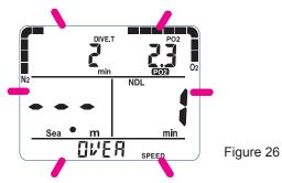
During an Out of Measurement condition the entire display blinks.
