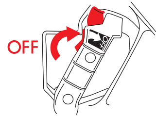
Main switch OFF
