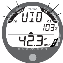
Fig. 41 - VIOLATION GAUGE MODE
