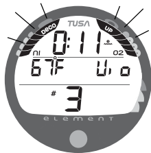
Fig. 46 - VIOLATION GAUGE MODE (Surface)
