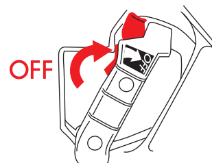
Main switch OFF
