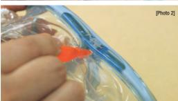
2 Use the plastic driver tip to pull the inner part prongs (which can be seen in Photo 1) from below, to remove the inner part. [Photo 3]
