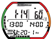
LOG-Decompression stop violation
